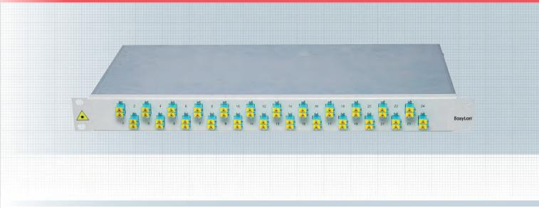
FO patch panel for fixed installation for up to 48 fibers. For SC / LC and LSH couplings the front panel is also supplied with screw holes in order to affix couplings. Cable entry is effected via a maximum of two cable glands or a fixture for break-out cable (each sold separately as special accessory). A breakout point is located on both sides on the back and serves as a holder for the FODH / FOCT distributor system.
